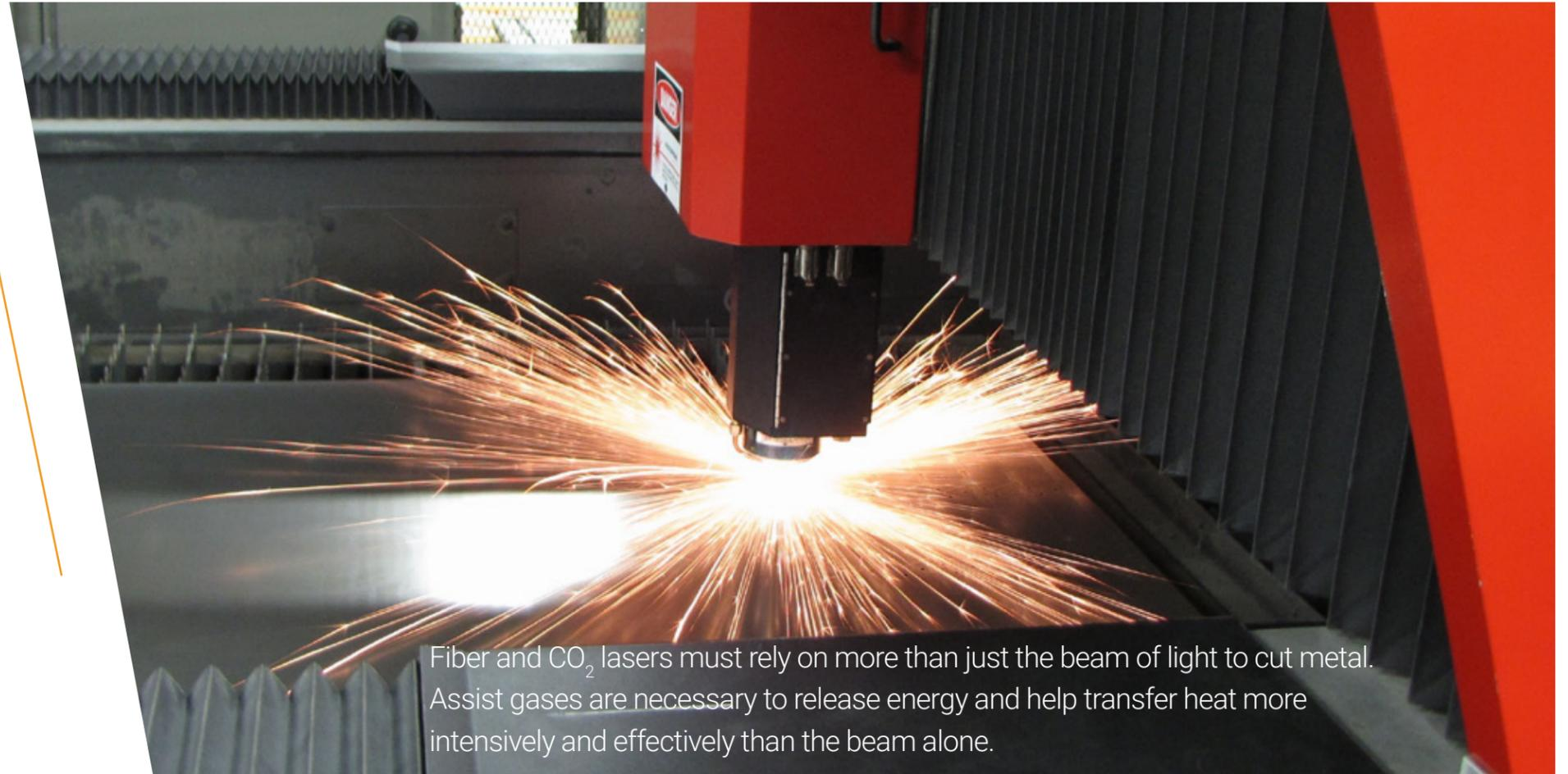
Fiber and CO<sub>2</sub> lasers must rely on more than just the beam of light to cut metal. Assist gases are necessary to release energy and help transfer heat more intensively and effectively than the beam alone.
