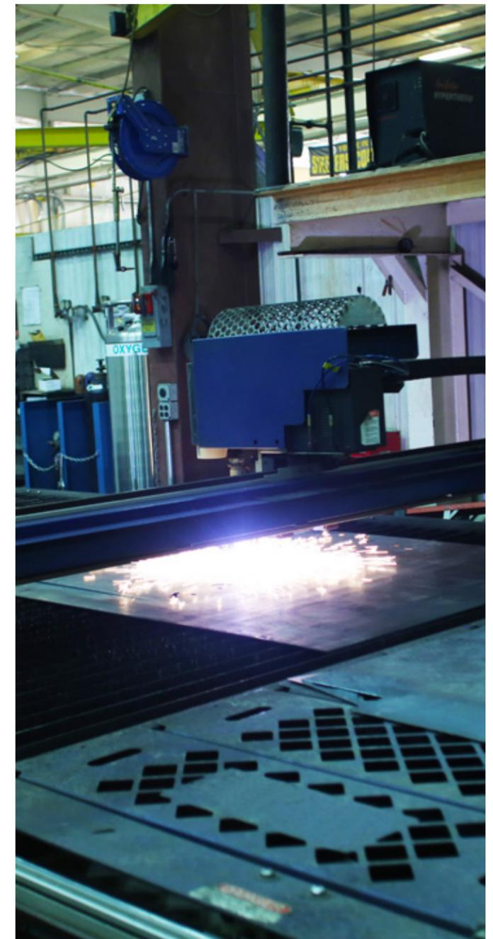
↑ When plasma and laser cutting fumes aren't properly removed from the air, measureable amounts of metals, such as hexavalent chromium, can build up in the bloodstream of those who are regularly exposed.
