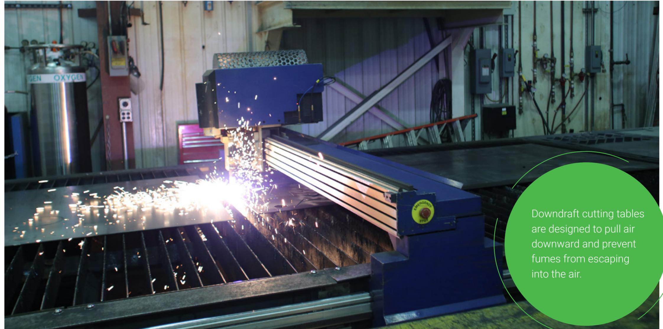
Downdraft cutting tables are designed to pull air downward and prevent fumes from escaping into the air.
