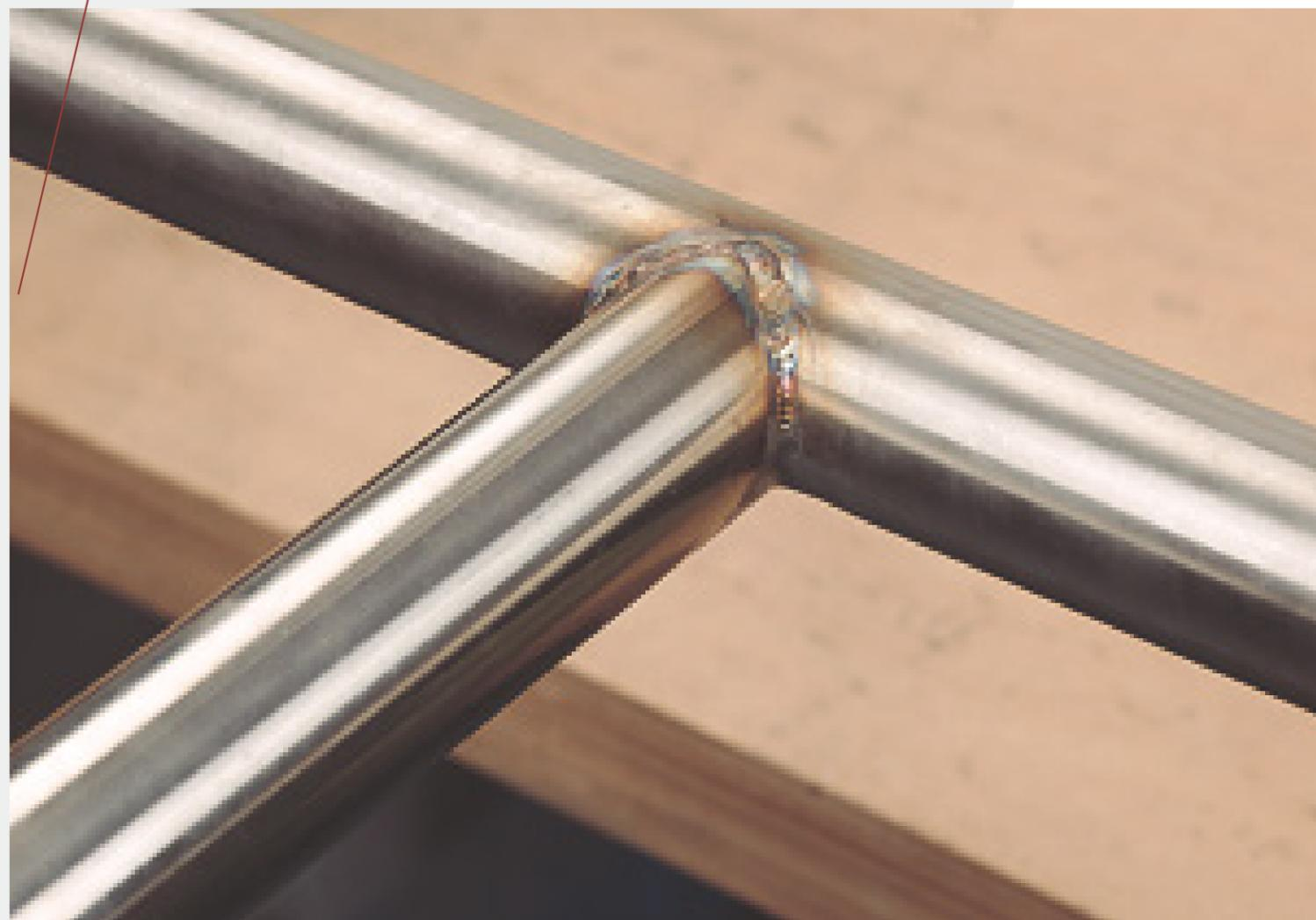
For flat surfaces, use an elastic drum and nonwoven nylon flat brush. For pipes and tubes, use a tube polishing wrap. Grain sizes to 320 will produce the desired results even on extremely small radii.
