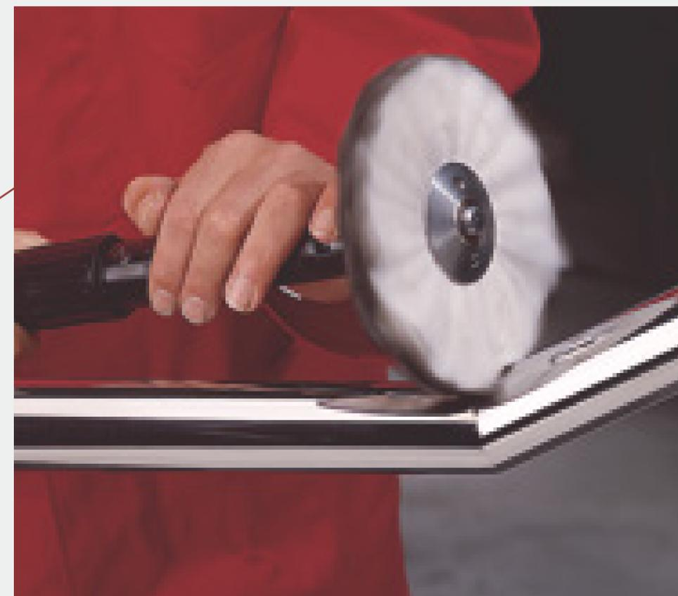
Fine grinding, by definition, is the blending of the weld to the surface of the metal for a smooth, consistent and attractive appearance. To produce the desired finishing results on stainless steel grades, there are a few tips that can help. And they often boil down to how today's handheld grinding equipment and consumables can affect a better outcome in a metals fabricating shop or manufacturing facility.
