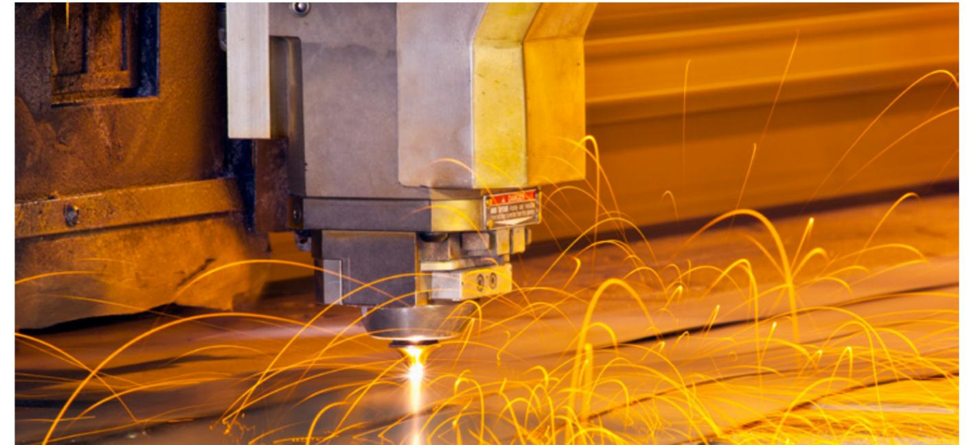
The amount of smoke produced by laser cutting depends on the thickness of the material, the length of the cut and the kerf, or width of the slit produced by cutting.
