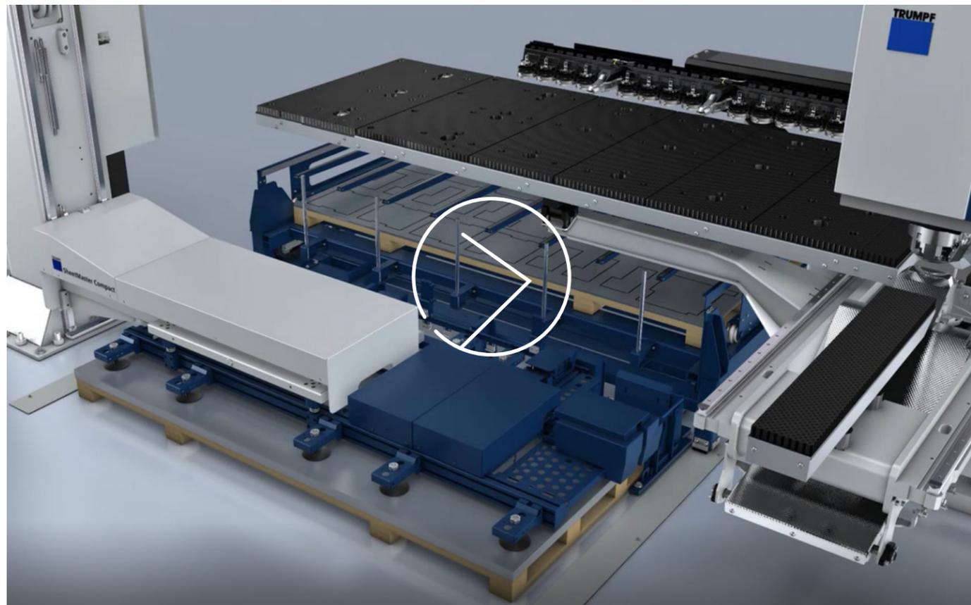
Trumpf's SheetMaster Compact offers an efficient automated way to load and offload material.
