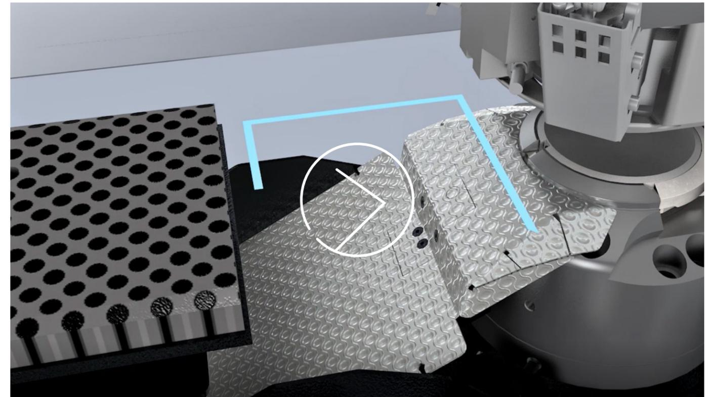
Watch how the TruMatic 1000 sorts parts and scrap into specific bins.
