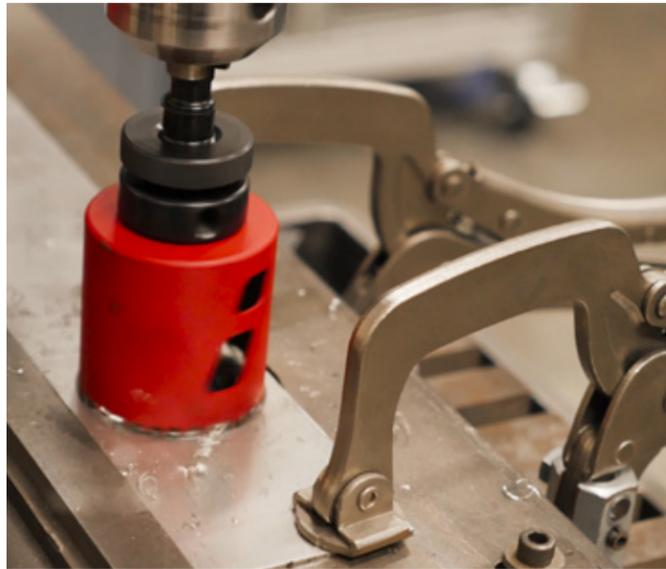
Selecting the correct cutting conditions (RPM and feed rate) is another essential approach for achieving better holesaw performance.
